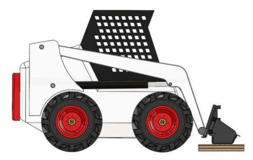
When the top edge of the coupler is seated in the top part of the coupler plate, roll the skid steer tilt function back until the attaching plate is flat against the skid steer coupler. Lock down the coupler levers. Note: If your skid steer is equipped with a hydraulically operated coupler, activate the coupler lock at this time.
